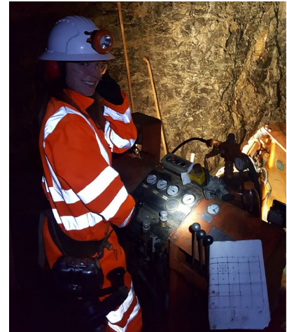
Face drilling with a single boom drill jumbo on a development heading underground at South Crofty. © Cornish Metals/Steve Tarrant
